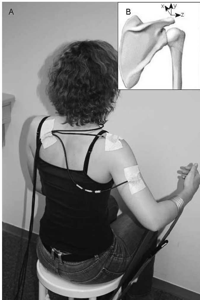
Figure 2. A, Receiver locations during 3-dimensional scapular position measurements. B, Coordinate axes for the local scapular reference frame.
